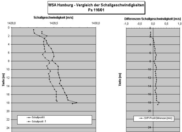
Fig. 1. Apparent comparison and difference calculation: comparison of sound velocities sound [sonic] velocity; differences; sound profile
