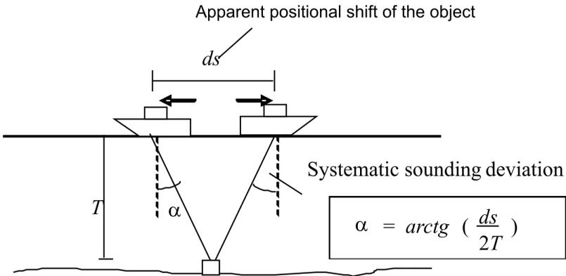
Fig. 3. On site testing of angle calibration
