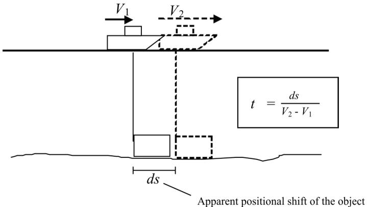
Fig. 2. Temporal assignment of the positioning system
