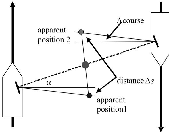
Fig. 4. Calibration in Multi Beam system
