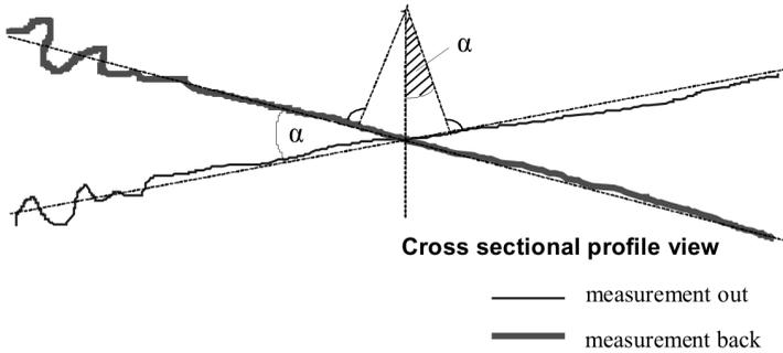
Fig. 5. Roll angle calibration
